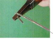
Take about five inches of the 21 gauge and, using your flat nose pliers, move up the jaw until the depth of one side of the jaw is the thickness of the two wire bundles just above the cabochon. Make a U bend in the wire. The short end should be slightly angled to allow for an even straight wrap around the bail.
